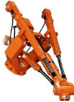
Figure (2.19): The ABB IRB940 Tricept Parallel Robot.
