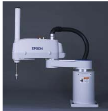
Figure (2.11): The Epson E2L653S SCARA Robot.
