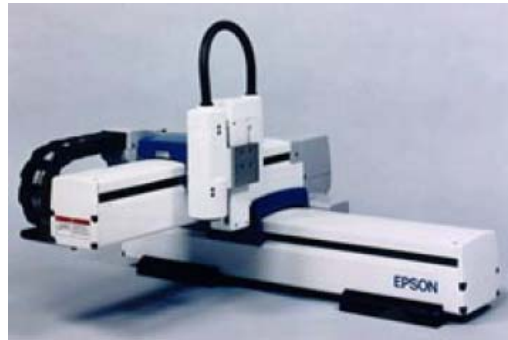
Figure (2.17): The Epson Cartesian Robot.
