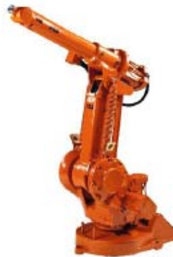
Figure (2.3): The ABB IRB1400 Robot.
